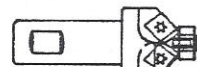
45° CHAMFER MILL WITH 1/2" SHANK #3/8 GUIDE BEARING WITH #3 SHCS USED IN A MANUAL ROUTER TO CHAMFER STEEL BY HAND
